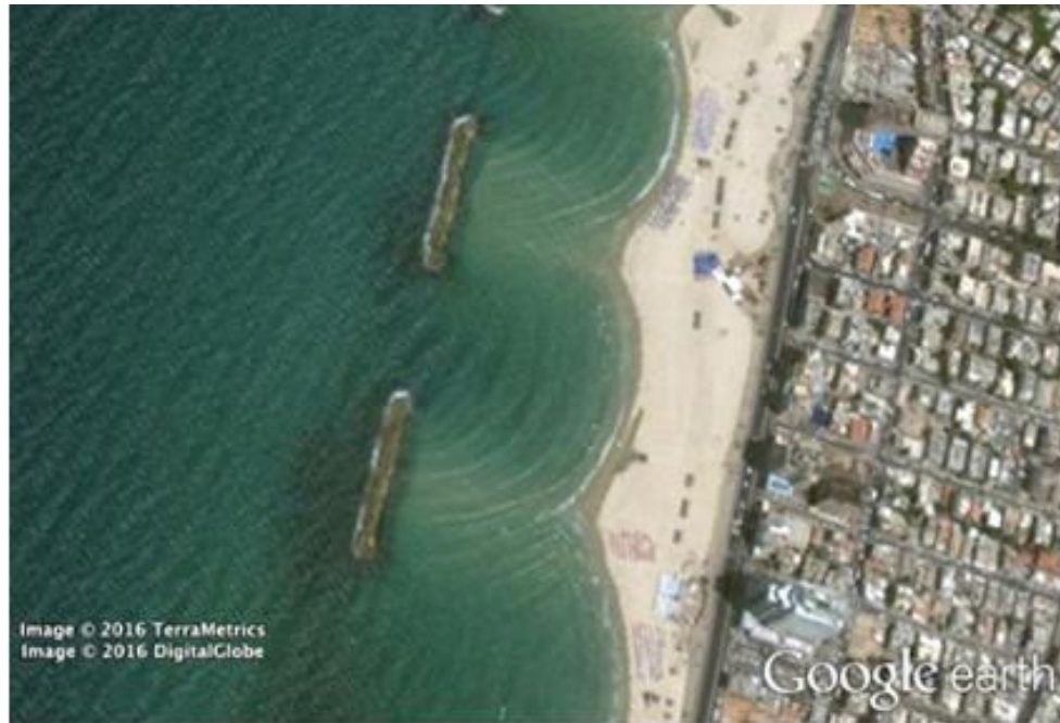
Figure 4.2 Because of the diffraction of waves, ocean waves entering through an opening in a breakwater can spread throughout the bay. (credit: modification of map data from Google Earth)
