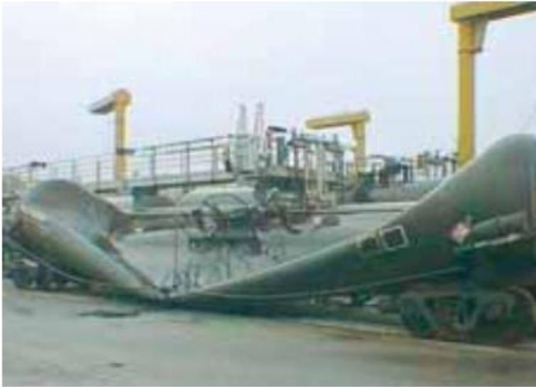
Fig. 19-1 A railroad tank car crushed overnight. (Photo courtesy www.Houston.RailFan.net )
